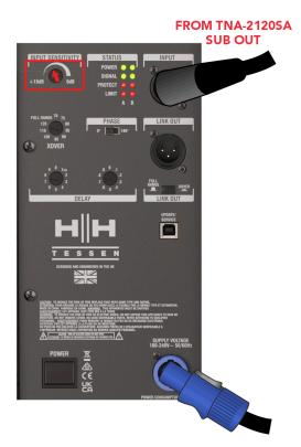
Connect the TNA-2800SA as above, from the line level sub-out of the TNA-2120SA, to utilise it as part of a full-range TNA system. Follow the power cycle instructions, and gradually turn the TNA-2800SA input sensitivity up to a suitable level, this should be around 10-11o'clock.
