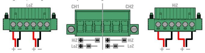
The speaker connector mode is determined by the type (HiZ Voltage / LoZ Impedance) for speakers connected and is configured by the settings of DIP switches 1, 2, 3 and 4 on the rear panel.
