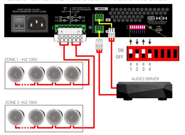
In this example, both channels are connected to high impedance ceiling speakers at 100V line level.
