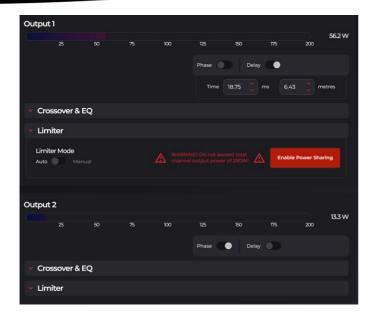
**OUTPUT** – View the status of both output channels. Various controls allow for customisation of peak & RMS limiters, Crossover, EQ and the ability to enable power sharing mode.
