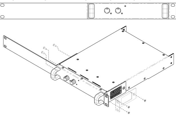
These are secured three M4 x 10mm CSK Head Machine screws per side.
