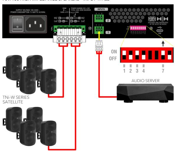
In this mode, the audio signal connected to CH1 Input will be routed to both CH1 and CH2 outputs. NOTE: CH2 Input is disabled, so even if a signal is connected, it will not be heard from CH2 Output.
