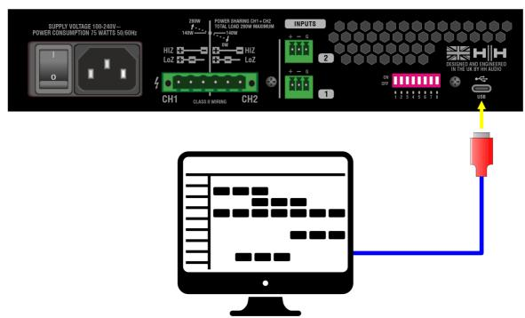
The MZ-140DX is equipped with a USB Type C port to allow for connection to a computer.
