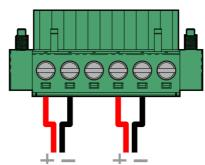
Make sure to check the combined impedance of all the speakers you are connecting to the output channel - this should be equal to (or more than) the LoZ setting (4 or 8 Ohm) that it's set to.
