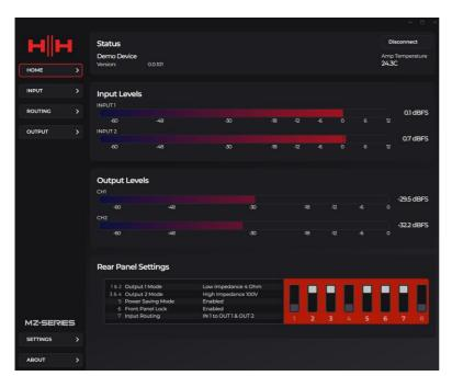
HOME – Provides a brief overview of the current status of the MZ-140DX. Including input and output levels and current DIP switch settings.
