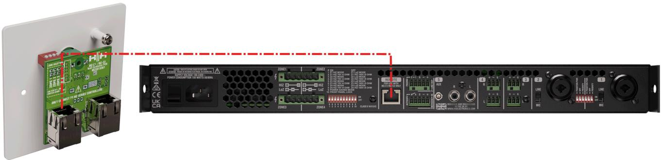
If multiple wall controllers are required, they must be connected in daisy chain formation from one to the next. Do this by connecting the **OUT** of the previous controller to the **IN** of the next via an RJ45.
