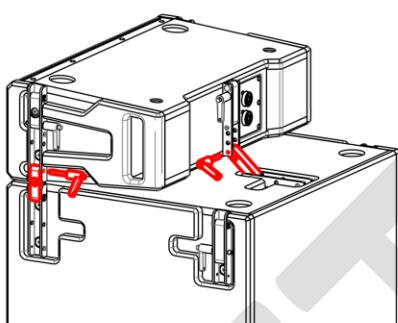
Rotate the pin mechanism to align with the mounting hole on the TNA-2051-G3
