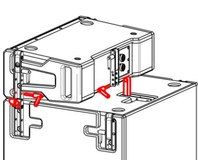
Push to release the locking pin on the sub and remove.
