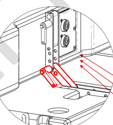
Angle adjustment is achieved with the rear locking pin and location holes.
