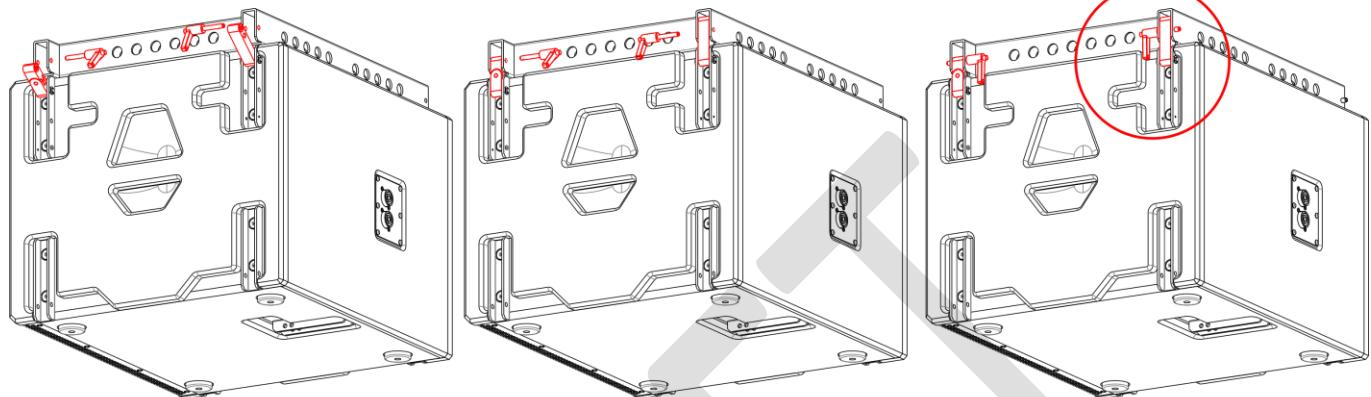
Push to release the locking pin on the sub and remove.
