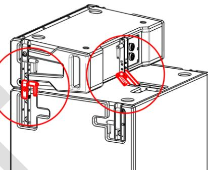
Press the locking pin button then insert into the bracket ensuring it is all the way home. Repeat with the remaining side locking pin.
