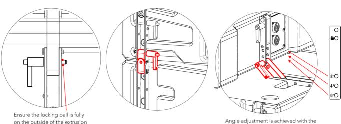
on the outside of the extrusion and check it is secure. Pull to check.
