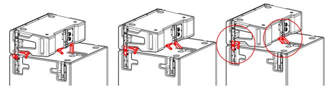
Push to release the locking pin on the sub and remove.
