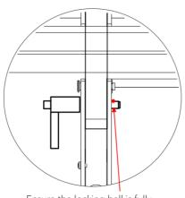
Ensure the locking ball is fully on the outside of the extrusion and check it is secure. Pull to check.
