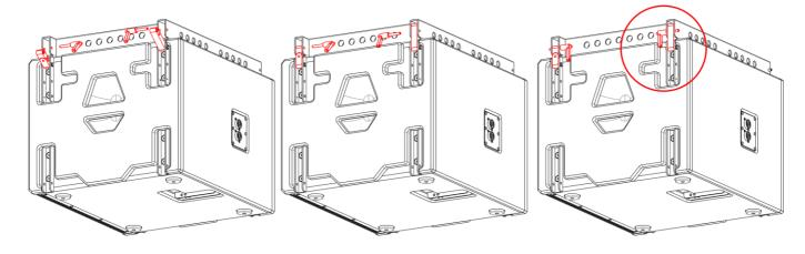
Push to release the locking pin on the sub and remove.
