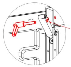
For the two rear fixing, the BOTTOM hole on pivot pin must be used.
