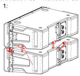
Push to release the locking pin and remove.
