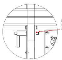
Ensure the locking ball is fully on the outside of the extrusion and check it is secure. Pull to check.
