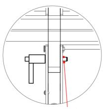
Ensure the locking ball is fully on the outside of the extrusion
