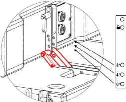
Angle adjustment is achieved with the rear locking pin and location holes.
