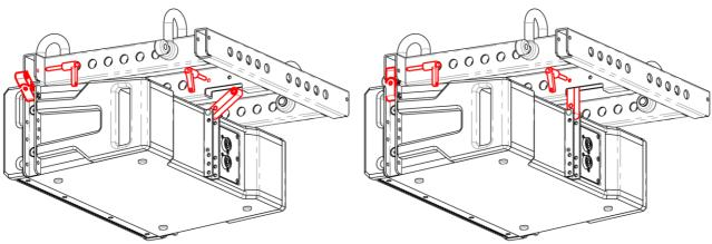
Push to release the locking pin on the sat and remove.
