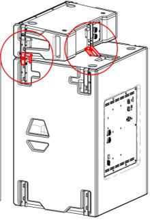
Press the locking pin button then insert into the bracket ensuring it is all the way home. Repeat with the remaining side locking pin.
